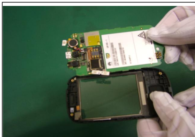
8. Remove the PCBA from the front cover.
