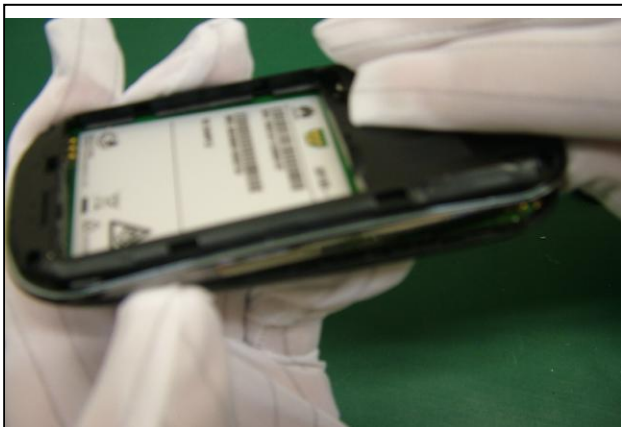
5. Release the latches between front and rear covers.
